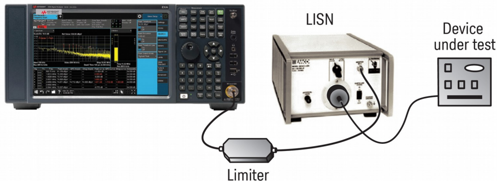
X-Series analyzer with N6141C EMC measurement application
